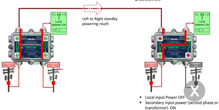
The second alternative power is from a distant available source over existing coax or power cable (typical from the remote Main electricity Tower and different network) using the two-way powering route on the same cable - patented technology
