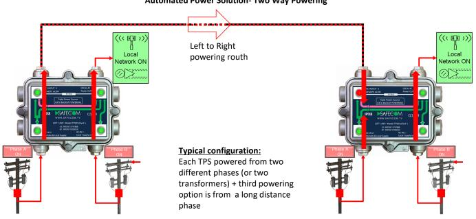
In the event of a power outage at local Power Supply AC1 the TPS Grid Controller first priority draws power from adjacent phase connected to AC2 input port (probably next electric pole & transformer)
